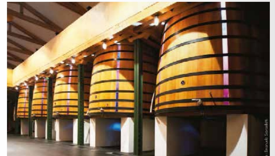
Seguin Moreau created tanks with transparent staves for Château Mouton Rothschild. The see-through staves allow winemakers to view fermentations in action.
